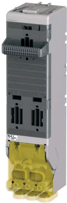
SLD 1 Fuse-switch-disconnector. - AC-23B according to IEC 60947-3 at 400 V. - 10 modules or 120 mm width. - Fuse NH 1 (max width 42 mm).
